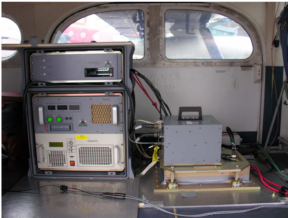
Optech ATML 3100 Scanner Head installed in PC-6 MSN 935 (HB-FMP)
