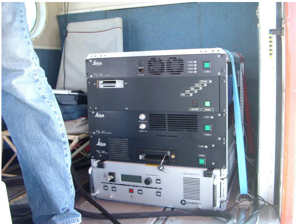
MM 40 Mass Memory with 540 GB installed in MSN 877 (HB-FPK)
