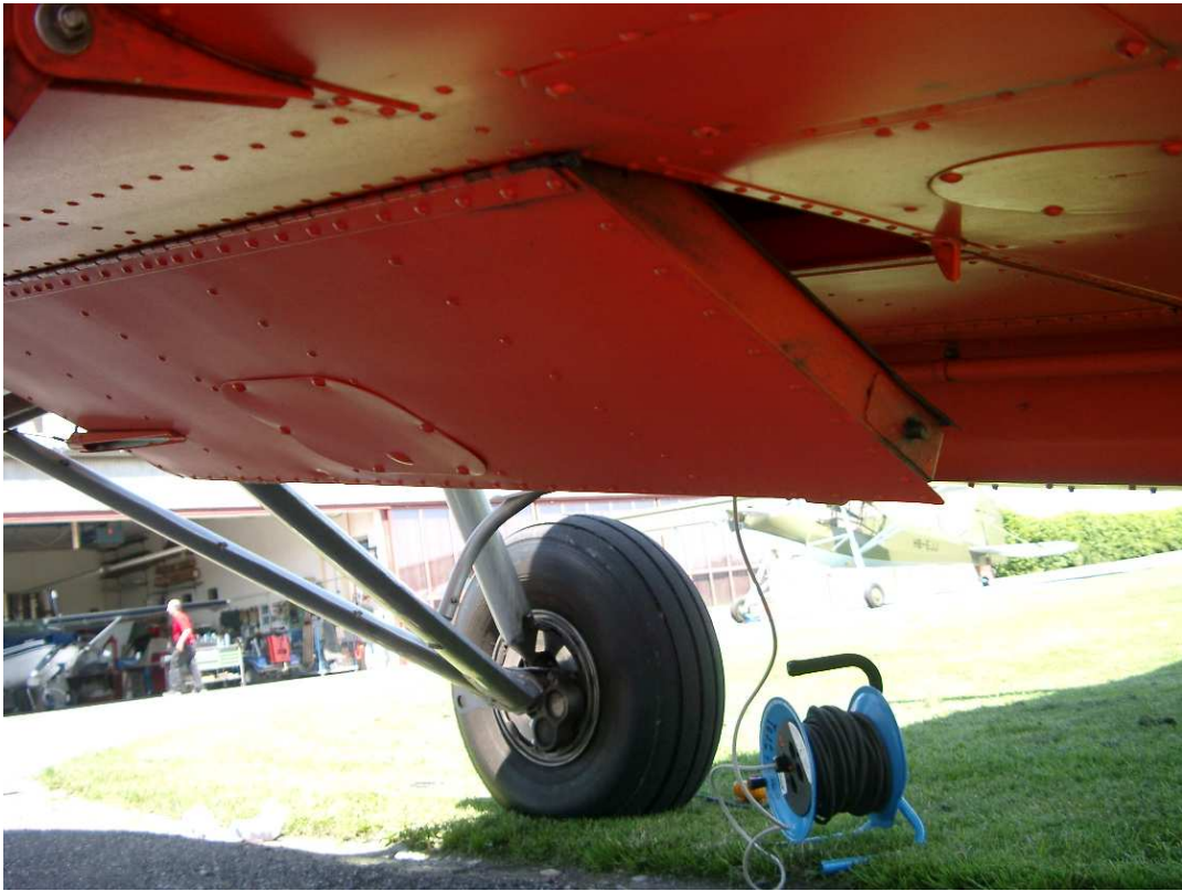
Trap Door start to opening
